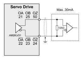
Example of encoder output signal, high-speed optocoupler.
