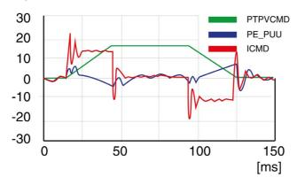
Example P8-20 (NLPEAFF) negative position deviation during acceleration phase (100 Hz)
