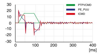
Step 7: Compensation of the Flexibility of the Mechanical System
